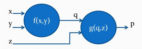
$$\frac{\partial p}{\partial x} = \frac{\partial p}{\partial q} \frac{\partial q}{\partial x}$$
